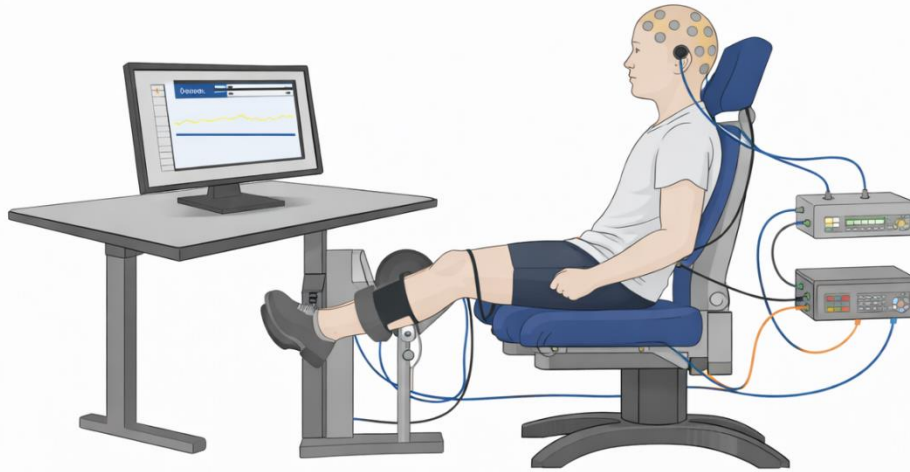
Figure 1. Experimental setup and task protocol. Schematic representation of the unilateral isometric knee flexion task. Participants were seated with the hip flexed at approximately 90° and the knee fixed at a constant flexion angle. The lower limb was secured to an isometric dynamometer, and visual feedback of force output was provided to maintain a steady submaximal contraction. EEG and EMG signals were recorded simultaneously during the plateau phase of each trial.
